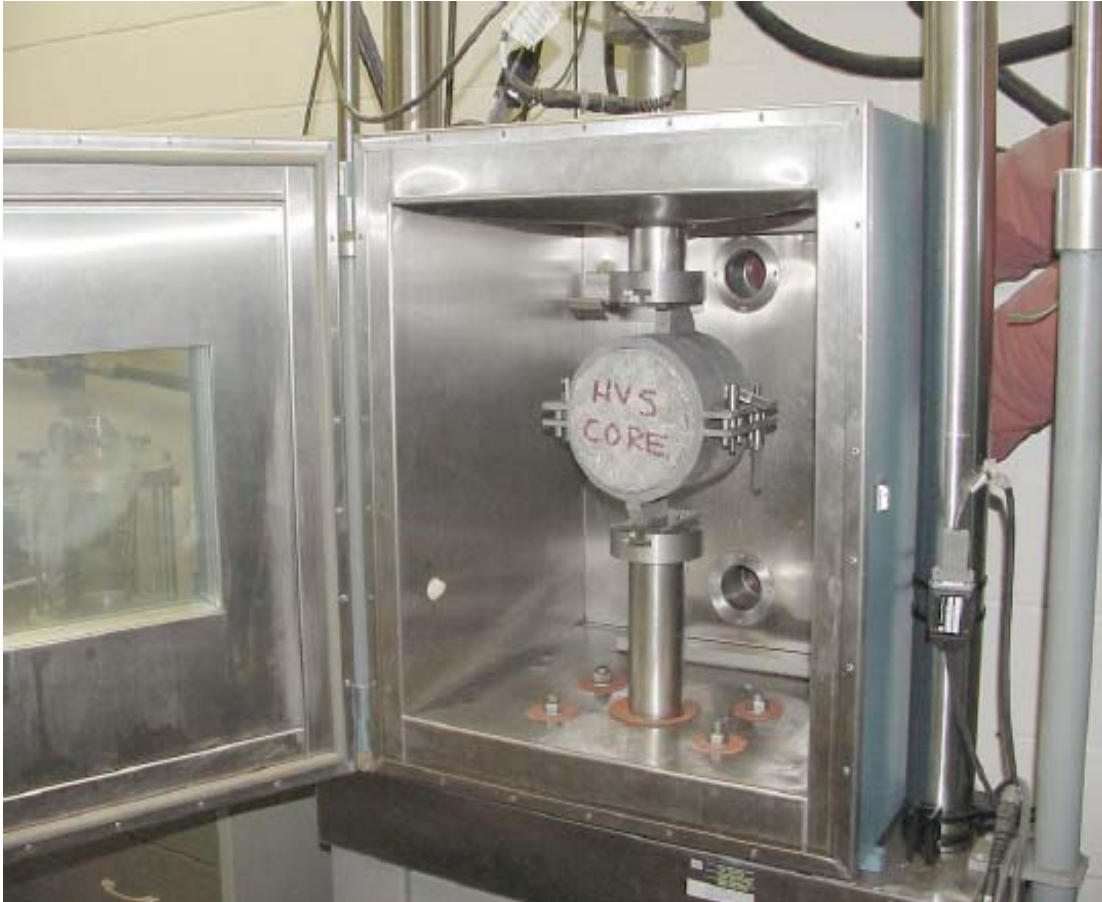
FIGURE 18 Shear Measurement Setup Developed by FDOT (17)
