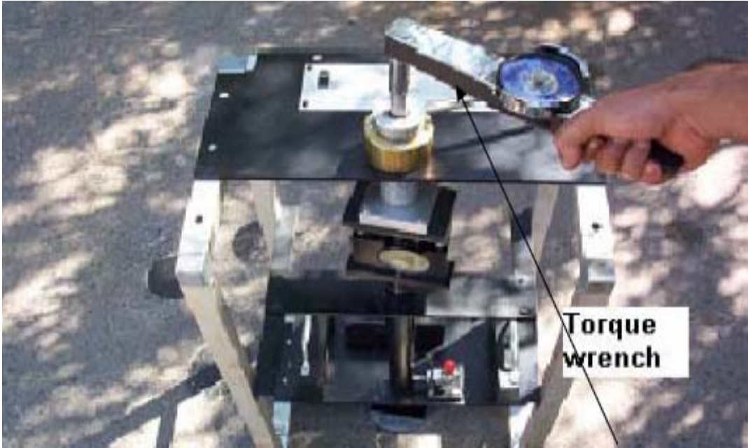
FIGURE 7 ATACKer™ Shear Strength Measurement With Torque Wrench(17)
