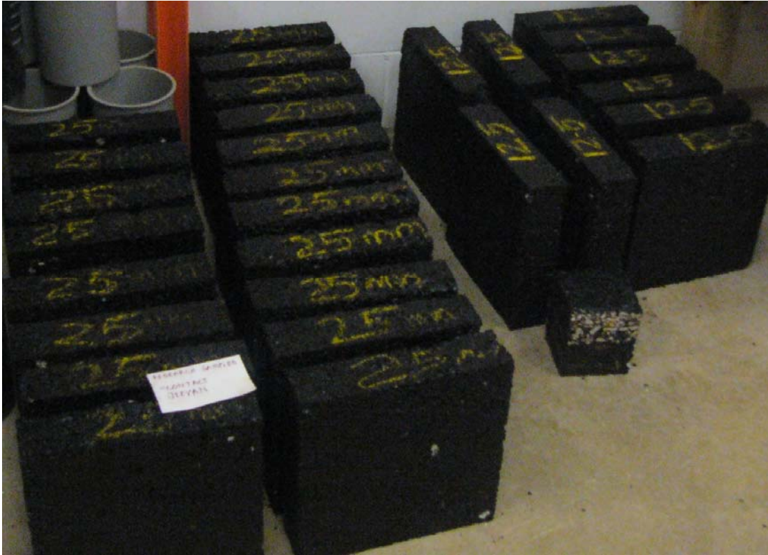
FIGURE 22 Compacted Bottom Slabs
